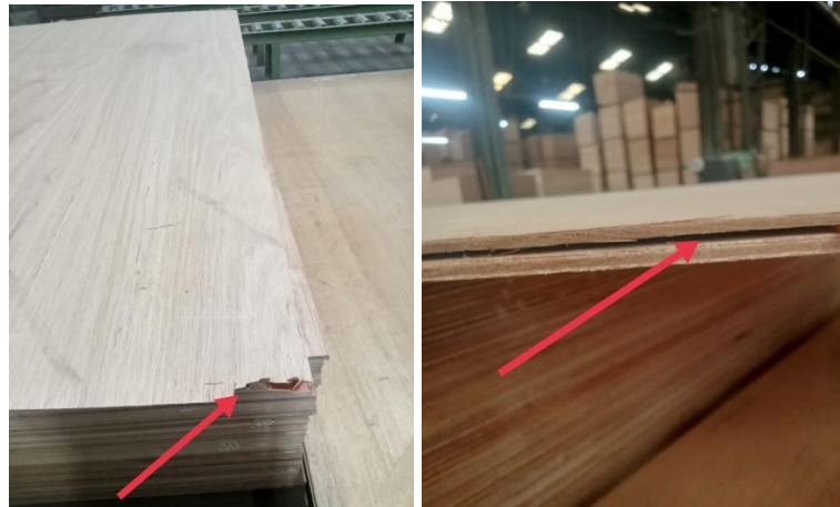
Gambar 1.2 Waste defect kayu plywood
